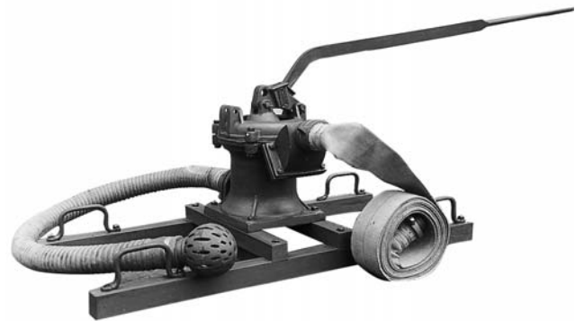
Fire Extinguishing Pump around 1930.
